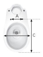
A - Dimension between the centre of each hole (mm)
